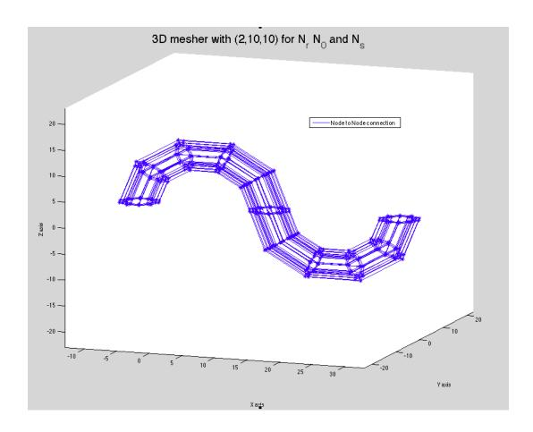
For this mesh, only element connectivity is shown, for the star plotting became visually obstructive:
